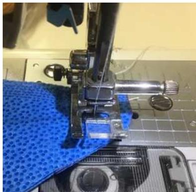
Presser foot position for **inner** seam with the needle centered.
