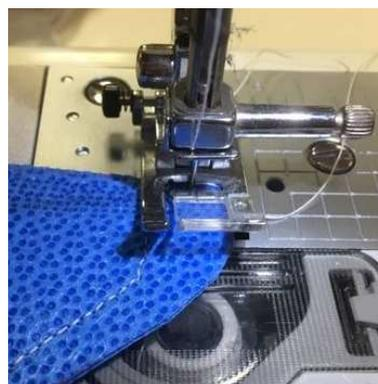
Presser foot position for **outer** seam with the needle centered.
